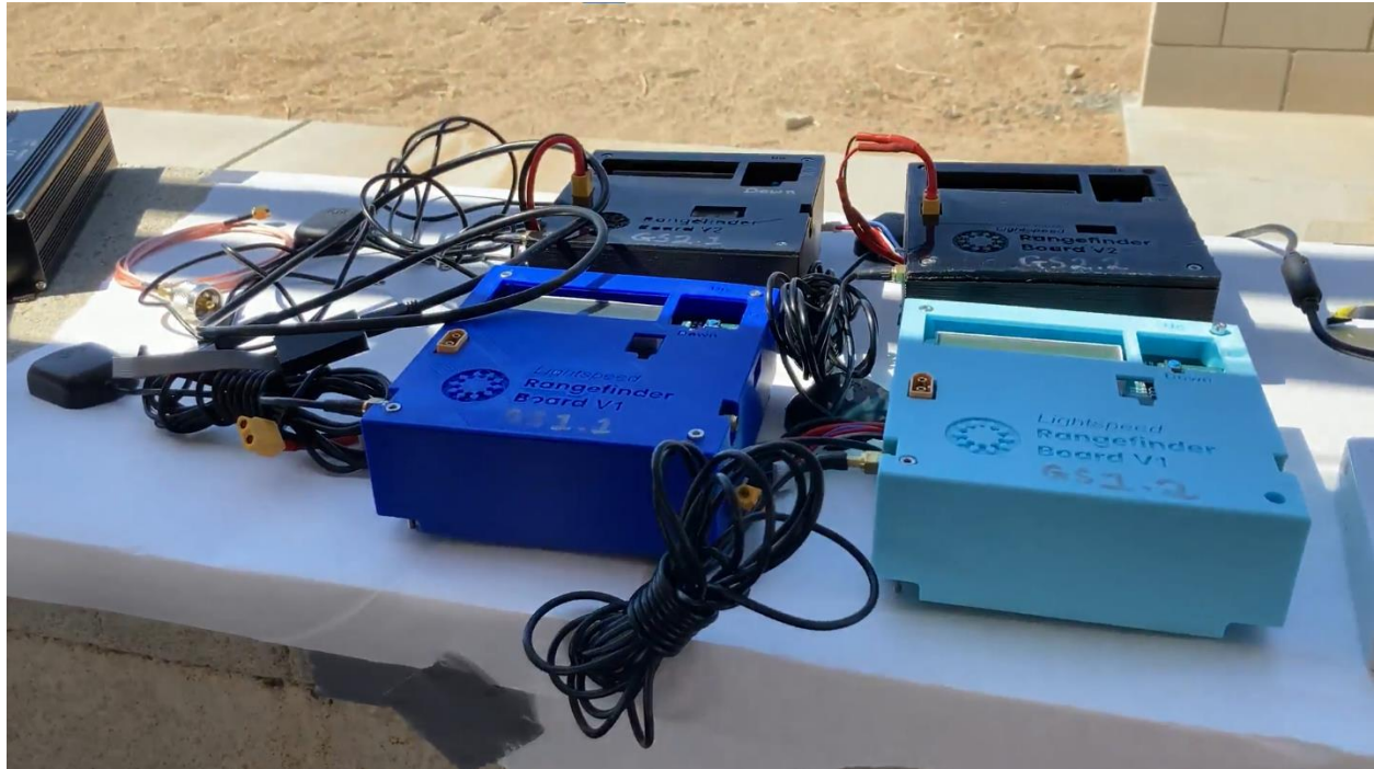
Figure 3.21. Four beautiful, completed rangefinder ground stations.
