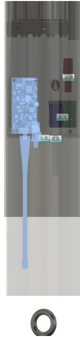
Figure 4.7.4. Rangefinder unit (highlighted) next to the XBee radio in the CAD for Lumineer.
