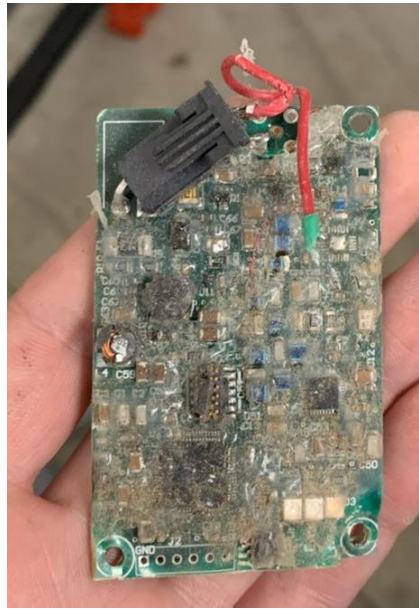
Figure 4.7.3. Transponder PCB after recovery from the crashed vehicle. Note that prior to flight the PCB was coated in silicone potting compound to protect it from G-forces and condensation.
