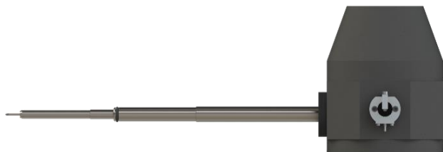
FIG. 1. Miniature high-vacuum valve attached to the dewar of a cryo-electron microscopy holder.
