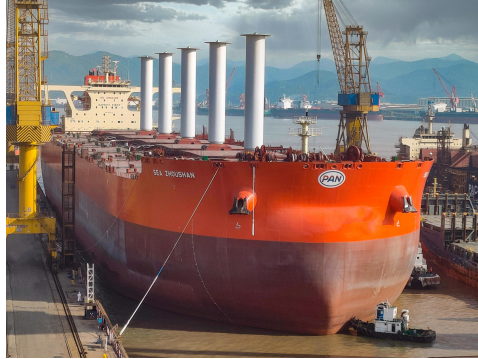
Figure 1: Very large ore carrier (VLOC) M/V Sea Zhoushan of the Brazilian mining company Vale, equipped with five rotor sails. Pictured in Zhoushan, China April 29, 2021. Credit photo: Vale.
