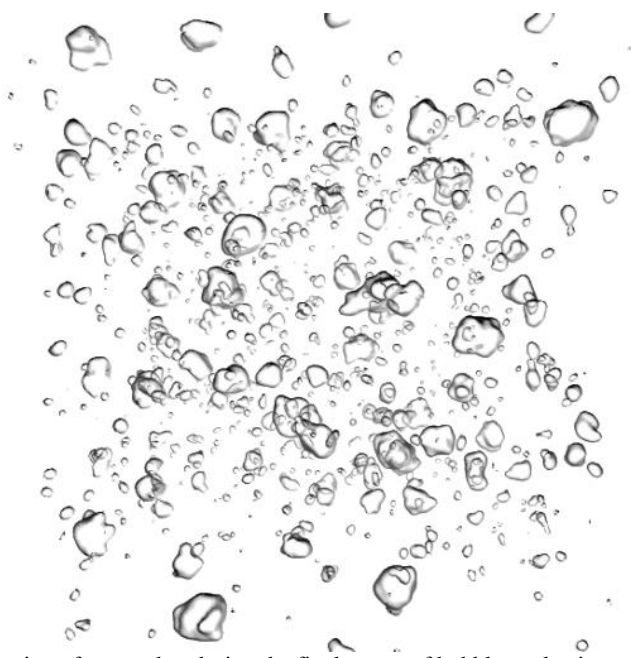
FIG. 1. Iso-density surface representation of a snapshot during the final stages of bubble nucleation at T = 280 K and \rho^h = 17.2 mol l -1 . The surfaces are generated by Gaussian density mapping using the quicksurf algorithm 51 in vmd 52 and mark aggregations of unit cavities as defined in paragraph III.A.
