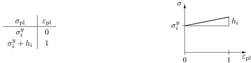
Figure 13: Realization of plastic hardening in Abaqus: Relation between plastic strains  $\epsilon_{pl}$  and stresses  $\sigma_{pl}$  for each interface layer  $i = 1, \dots, 4$ .
