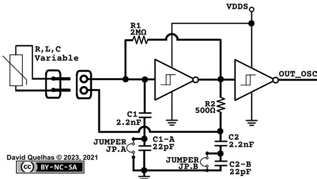
Figure 2: Schematic of the sensor interface circuit (oscillator).
