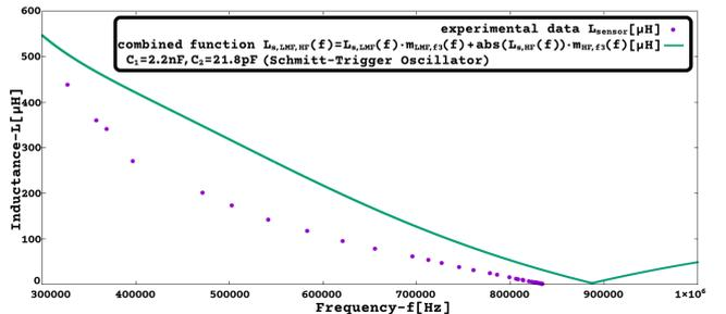
Figure 32:  $L_{s,LMF,HF}(f)$  [ $\mu\text{H}$ ], frequency in [300kHz, 1MHz] (Sch-trig. osc., Multi-Sensor Int. with inductive sensor, LMF and HF combined approx. function, with  $C_1=2.2\text{nF}$ ,  $C_2=21.78\text{pF}$ ).
