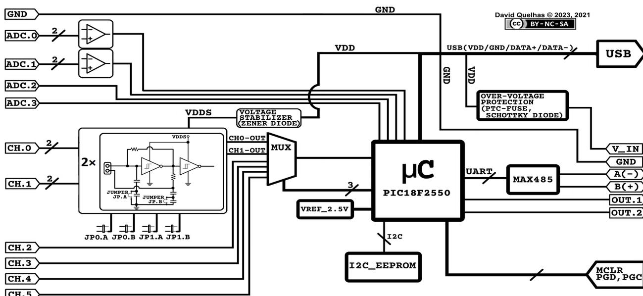
Figure 1: Diagram of the Multiple Sensor Interface device.
