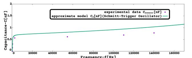
Figure 23:  $C_s(f)$  [nF] by approximate model, frequency in [0Hz, 170kHz] ( $C_{approx}$ ,  $R_{approx}$ ; Multi-Sensor Int. with capacitive sensor)
