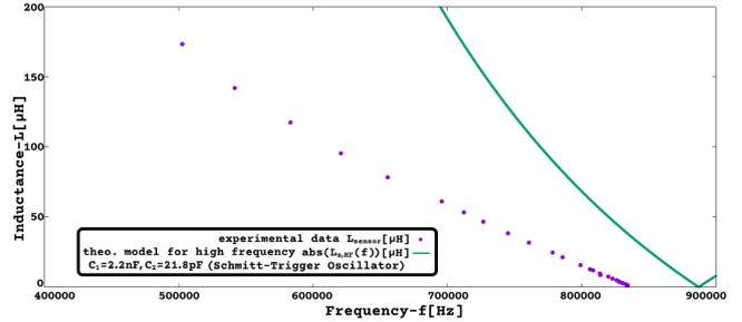
Figure 27:  $abs(L_{s,HF}(f))$  [ $\mu$ H], frequency in [400kHz, 900kHz] (Sch-trig. osc., Multi-Sensor Int. with inductive sensor, HF approx. function).
