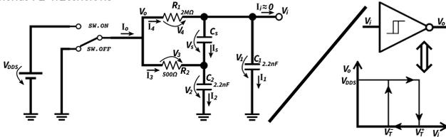
Figure 13: Multi-Sensor Int., capacitive sensor (Schmitt-trigger osc.)
