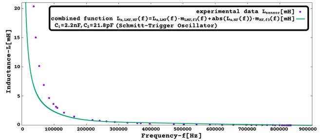
Figure 31:  $L_{s,LMF,HF}(f)$  [mH], frequency in [0Hz, 900kHz] (Sch-trig. osc., Multi-Sensor Int. with inductive sensor, LMF and HF combined approx. function, with  $C_1=2.2\text{nF}$ ,  $C_2=21.78\text{pF}$ ).
