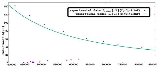
Figure 8: Frequency jump of  $L_s(f)$ [ $\mu H$ ]([Hz]) with  $C_1=C_2=2.2nF$  (Pierce osc., Multi-Sensor Int. with inductive sensor).
