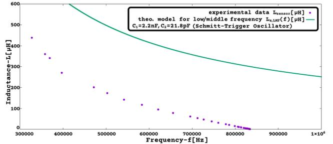
Figure 29:  $L_{s,LMF}(f)$  [ $\mu$ H], frequency in [300kHz, 1MHz] (Sch-trig. osc., Multi-Sensor Int. with inductive sensor, LMF approx. function).
