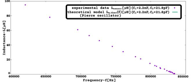
Figure 10: Experimental data of  $L_{sensor}$  in  $[0\mu H; 100\mu H]$ , with  $C_1=2.2nF, C_2=21.78pF$  (theoretical  $L_s(f)$  as a Pierce osc. is out of plot range).
