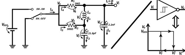
Figure 24: Multi-Sensor Int., inductive sensor(Schmitt-trigger osc.)
