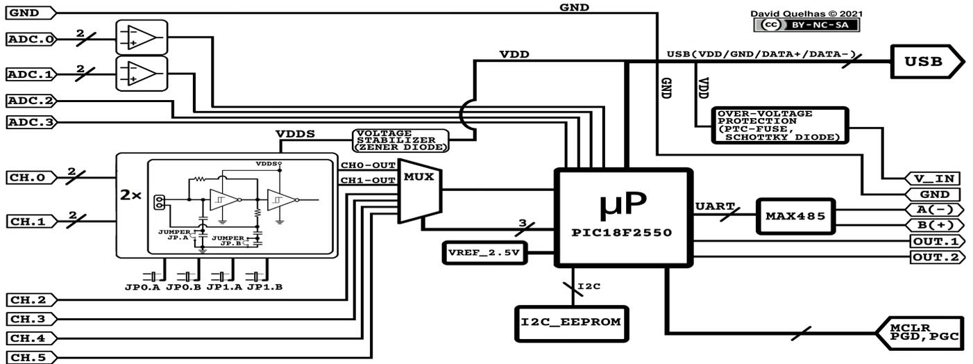
Figure 1: Diagram of the Multiple Sensor Interface device.
