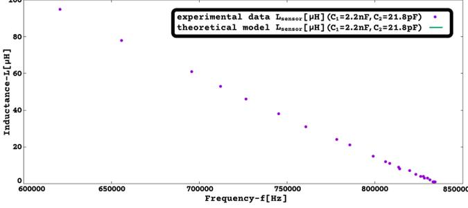
Figure 13: Experimental data of  $L_s$  in  $[0\mu\text{H};100\mu\text{H}]$ , with  $C_1=2.2\text{nF}$ ,  $C_2=21.78\text{pF}$ (Multiple-Sensor with inductive sensor).
