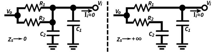
Figure 21: Schematic of the RC network of the Schmitt-Trigger Oscillator for the 2 extreme cases of the sensor impedance ( $Z_s$ ).
