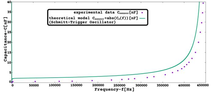
Figure 18:  $C_s$ [nF] versus frequency[0Hz, 450000Hz] by  $|C_s(f)|$  (Schmitt-Trigger Oscillator, Multiple-Sensor Int. with capacitive sensor).
