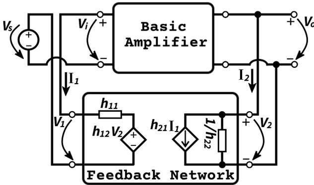
Figure 6: Representation of oscillator circuit by the h-parameters for feedback circuit (Pierce Oscillator).
