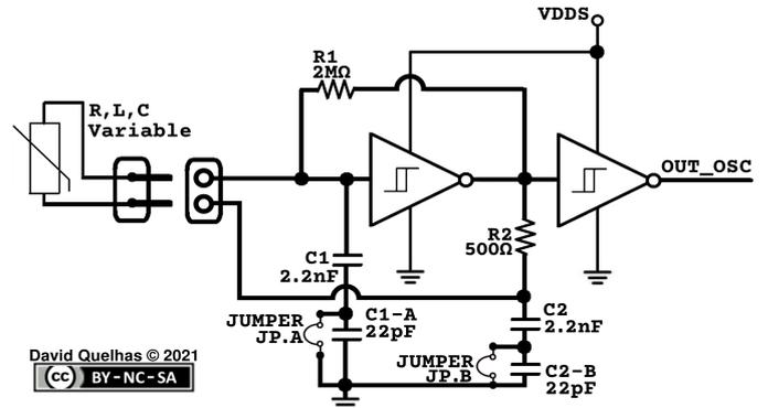
Figure 2: Schematic of the sensor interface circuit (oscillator).
