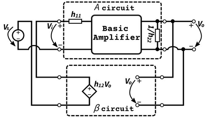
Figure 7: Simplified representation of oscillator circuit (Pierce Oscillator).
