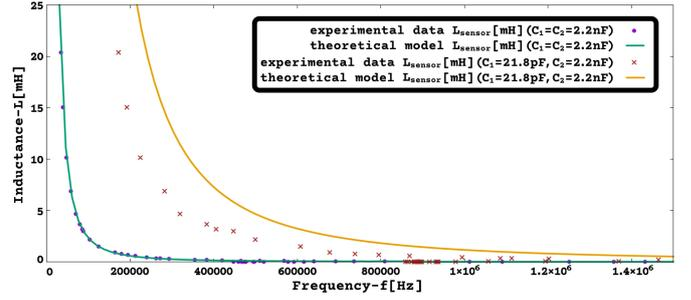
Figure 10:  $L_s(f)$ [mH]([Hz]) with  $C_1=C_2=2.2nF$  and  $C_1=21.78pF, C_2=2.2nF$  (Pierce Oscillator, Multiple-Sensor Int. with inductive sensor).
