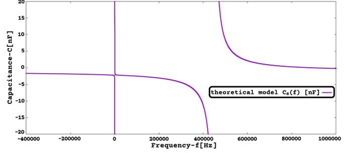
Figure 17:  $C_s(f)$  [nF] versus frequency[-400kHz, 1MHz] (Schmitt-Trigger Oscillator, Multiple-Sensor Interface with capacitive sensor). ( $f=0$ ), but also visible to the right is another curve that is also placed on the area of  $C_s > 0$  (for frequency[447957Hz, 895689Hz ] ) and at first this curve would be expected to define the operating frequency of the oscillator depending on the capacitance of the connected sensor.
