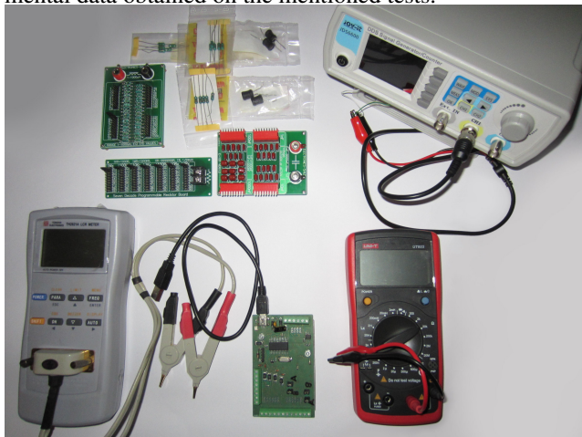
Figure 5: Equipment used for testing; R, C, L test components (top); and the Multiple-Sensor Interface (center bottom).
