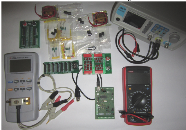
Figure 5: Equipment used for testing; R, C, L test components (top); and the Multiple-Sensor Interface (center bottom).
