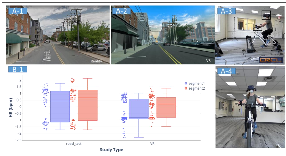
Figure 2. Comparison of real road(A-1) and IVE (A-2) environments; Video collection system of IVE bike simulator(A3-A4); Heart Rate Distribution of experiment(B-1)
