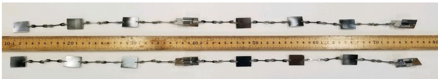
Figure 2. 316H sample chains that were hung in the vertical portions of the loop, one in the hot leg, and one in the cold leg.
