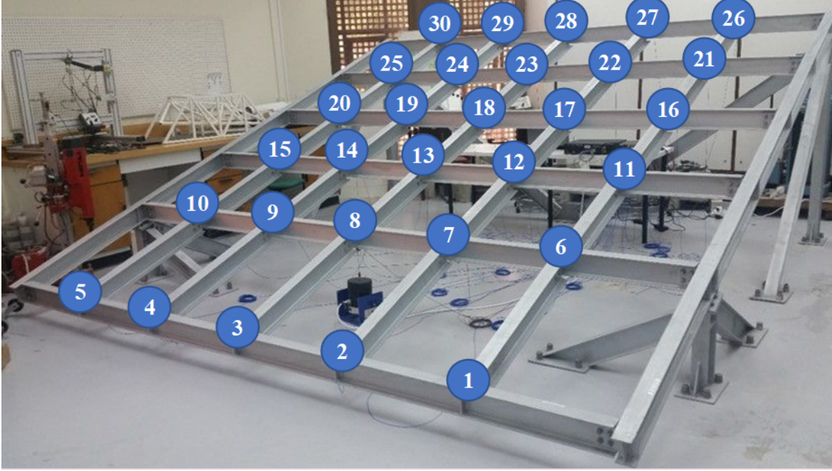
FIG. 4: QUGS testbed, where the joints are numbered from 1 to 30 (Abdeljaber et al. 2017). 35 36 37 38
