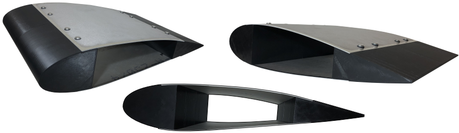
Fig. 16 The model of an airplane wing skin shaped as the NACA 5430 airfoil with a chord length of 500mm. The upper and lower skins were shaped using the shot peen forming, and the forward and the back parts (black) were printed in 3D. The structure is assembled using binding barrels and screws.
