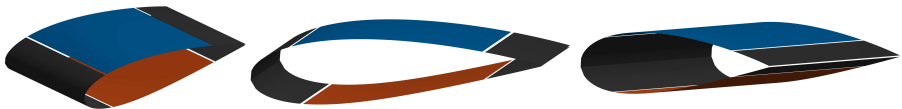
Fig. 10 The two target shapes for the 320 \times 320 mm sized panels made of aluminum 2024-T3. The target shapes constituted parts of the upper (blue) and lower (orange) airplane wing skins. The wing was shaped as the NACA 5430 airfoil with the chord length of 500 mm.
