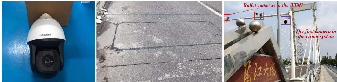
(a) Hikvision HD-Camera (b) MEAS Quartz WIM Sensor (c) Installed cameras on the bridge
