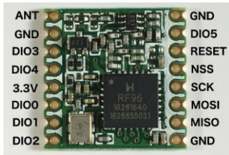
Figure 7. HopeRF RFM95W pin out
