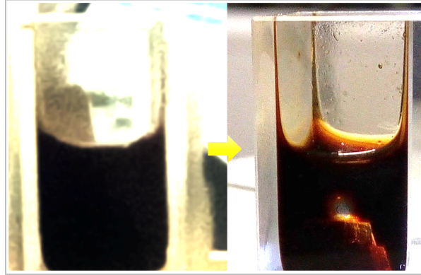
Figure 4. Comparing the glass beaker image (left) without using IRIDW and the appearance of the same beaker after using IRIDW setup (right), showing the first-ever image of a water droplet on top of calcite rock inside dark hydrocarbon fluid.
