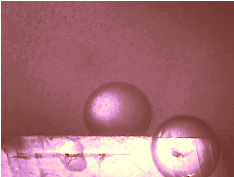
Figure 8. Image processing using digital filters to enhance the visibility of the water droplet on top of calcite inside a dark hydrocarbon.
