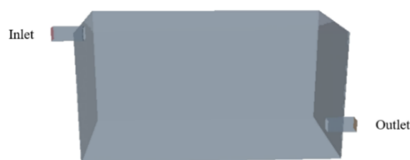
Figure 1: The room geometry to validate the computational model. Length: 0.8 \text{ m} , width/height: 0.4 \text{ m}
