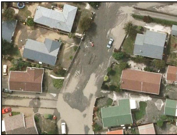
(c) Severe Liquefaction
