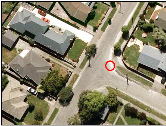
(a) Marginal Liquefaction
