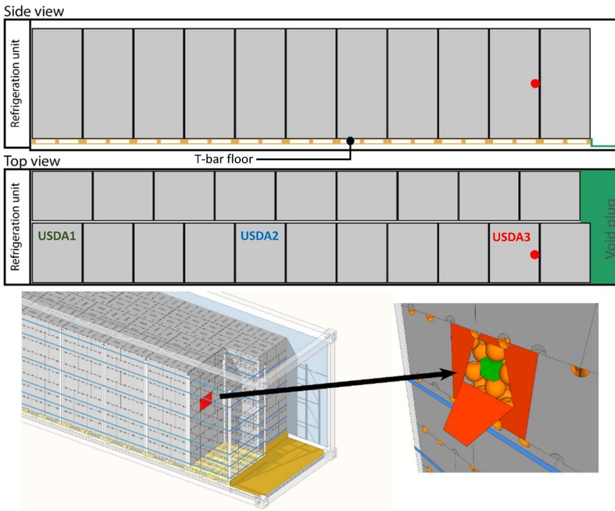
Figure S1. Side and top cross-sectional views of a refrigerated container with an indication of sensor placement.
