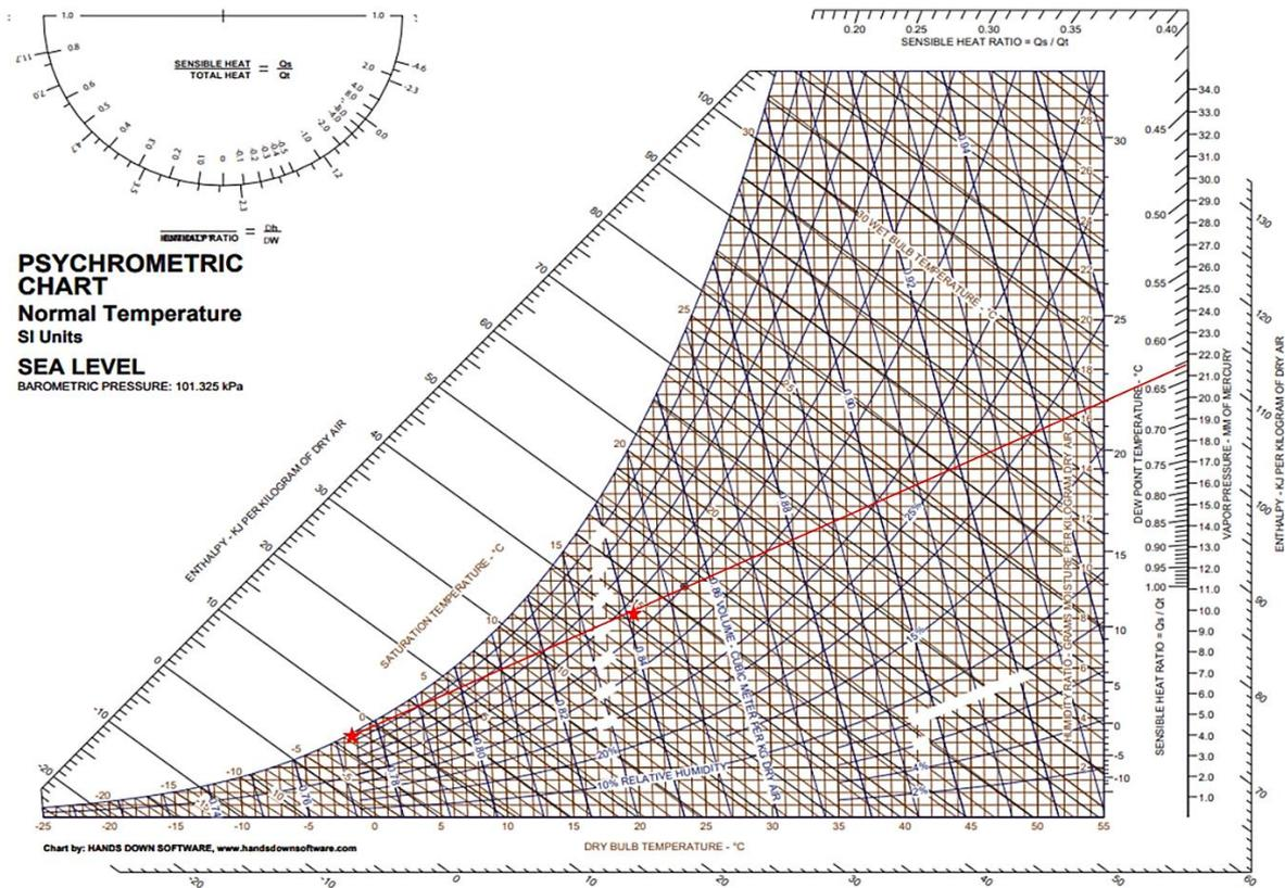
**Figure S2:** Psychrometric chart showing thermodynamic properties of the air in the refrigerated container as it transitions from ambient conditions ( $20^\circ C$ ,  $55\% RH$ ) to those of cold storage ( $-1.5^\circ C$ ,  $95\% RH$ ). This image is available in the public domain via (<https://chbe241.github.io/>).
