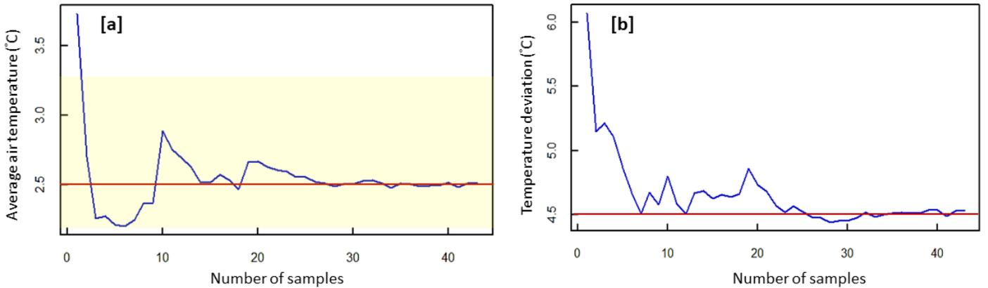
**Figure S3. Sample size analysis showing: [a] the relationship between average air temperature and number of samples, and [b] the corresponding deviation of the mean temperature from the final mean temperature. The red-colored straight line represents the final mean temperature, while the yellow-shaded area represents the accuracy range of  $1^\circ\text{C}$  for USDA approved temperature sensor.**
