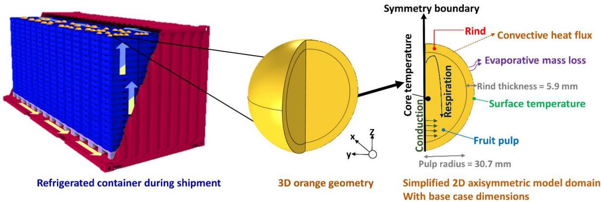
Figure 2. Geometry and boundary conditions of an orange in a refrigerated shipping container (figure not to scale).
