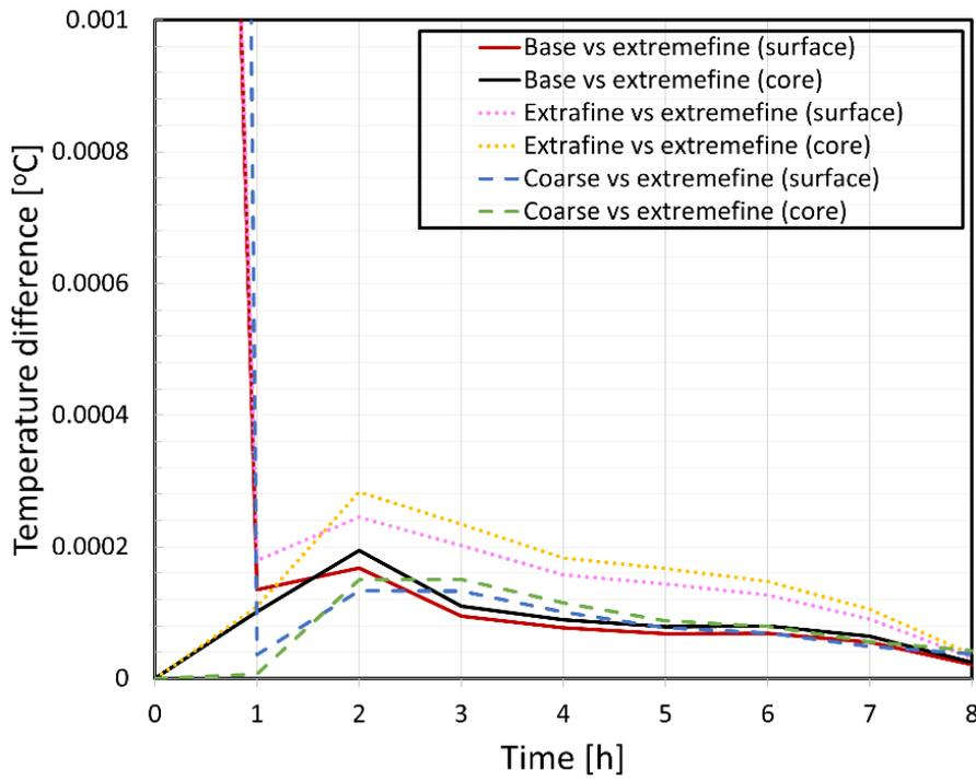
Figure S5. The difference in temperature of the base, extra fine, and coarse grid with the extreme fine grid as a function of time for the temperature at the surface and the fruit pulp core.
