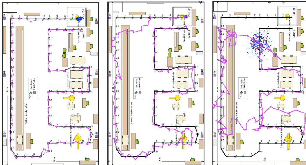
Figure 11. Decawave (left), BeSpoon (centre), Ubisense (right) accuracy comparison.
