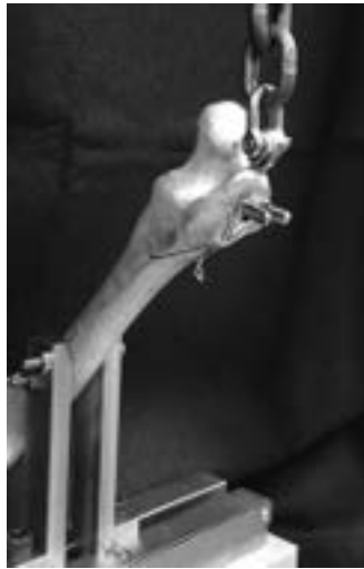
Figure 1. Solid brass right femur model with a 45° osteotomy, rigidly mounted in custom jig for mechanical testing of tension band configurations. Loads were applied via a steel chain at an angle of 45° to mimic gluteal tendon loading.
