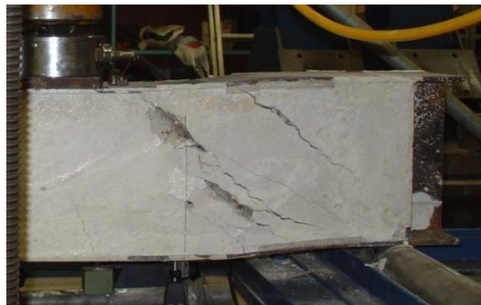
Figure 10. USFB No.4 at Failure point.
