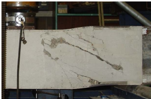
Figure 9. USFB No.3 at Failure point.
