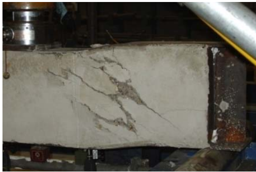
Figure 7. USFB No.1 at Failure point.
