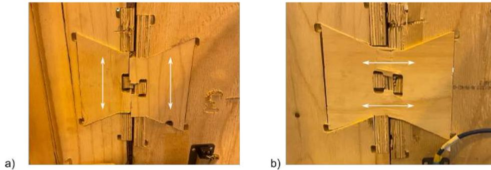
FIG. 8: Two possible grain orientations: a) 4 lamellae with grain parallel to the shear plane, 2) 2 lamellae with grain perpendicular to the shear plane.
