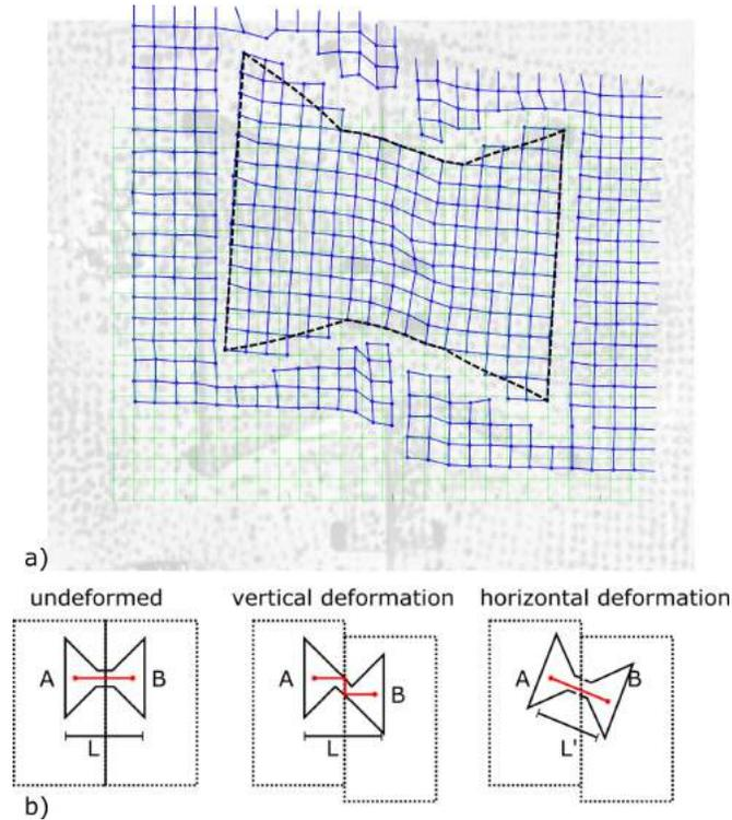
FIG. 11: Deformed shape of the shear keys: a) captured by using DIC analysis and b) conceptual behaviour.
