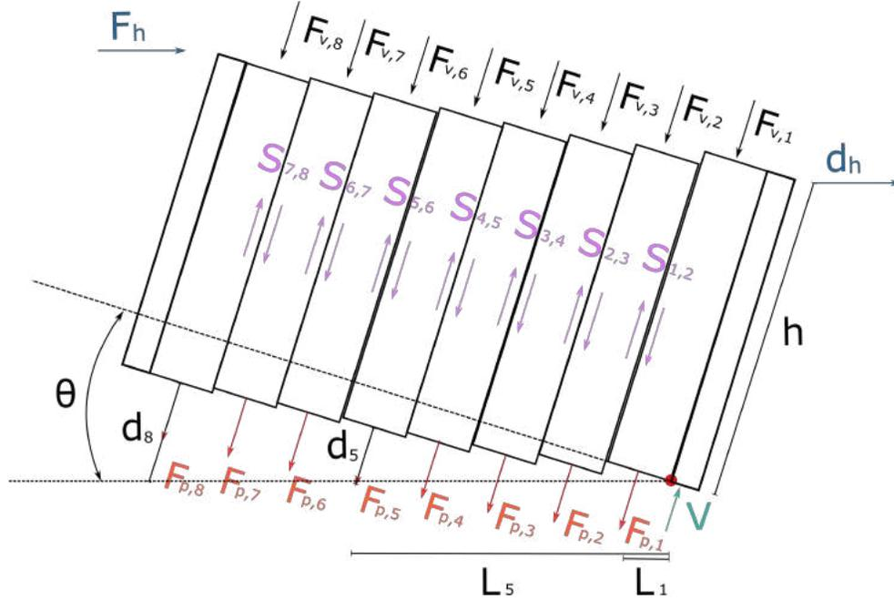
FIG. 15: Analytical model of the wall.
