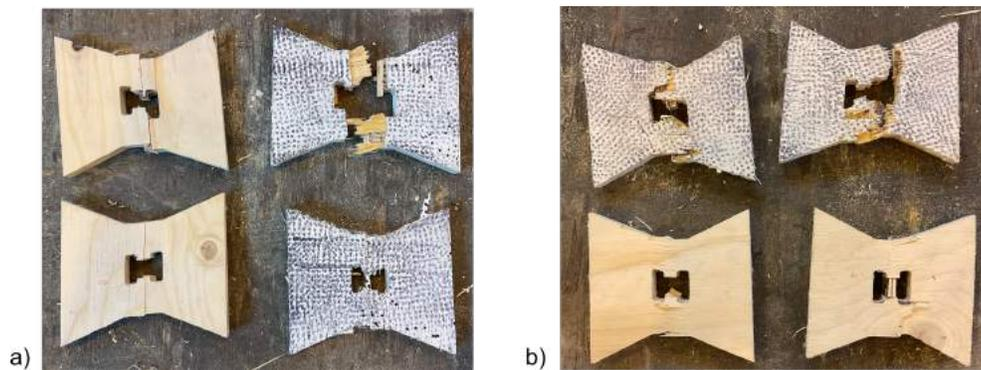
FIG. 10: Observed failure modes in the: a)  $PLY \updownarrow$  specimens, b)  $PLY \leftrightarrow$  specimens.
