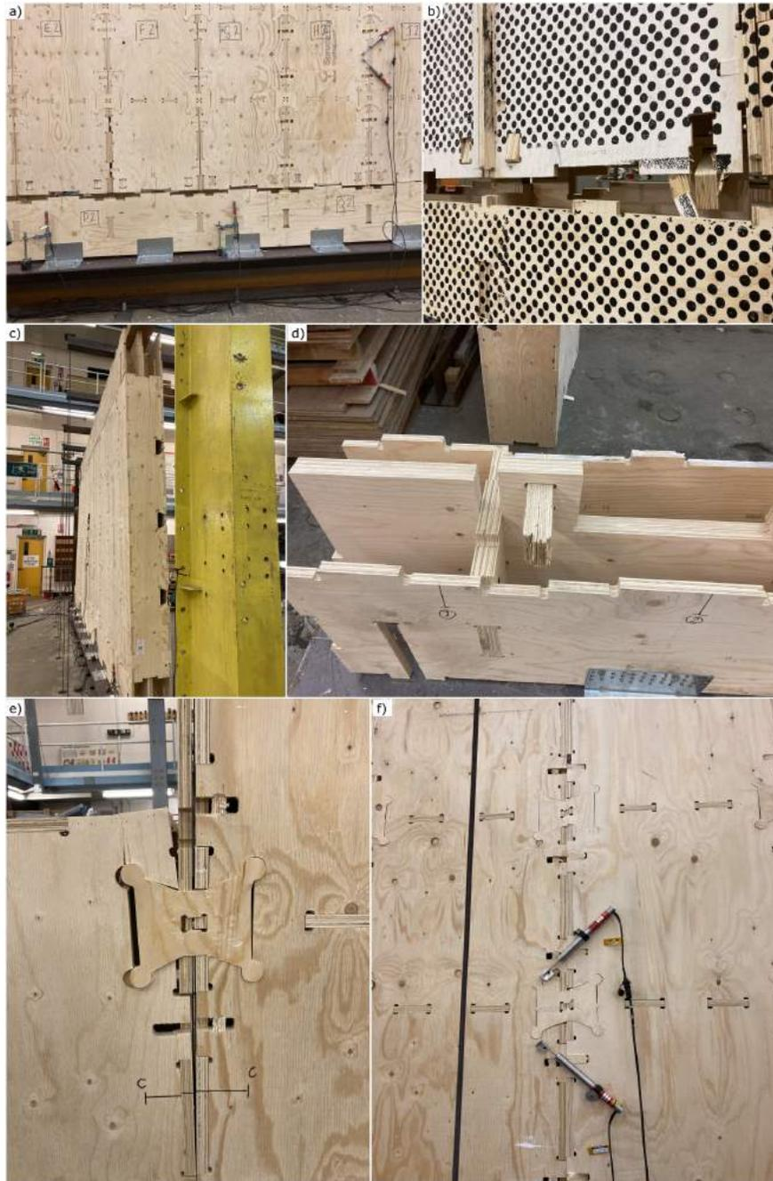
FIG. 5: Failures observed in the specimens: a) b) pegs failure in the SW\_noLoad specimen, c) out of plane bending in the SW\_Load specimen, d) pegs failure and e) splitting in the WW\_noLoad specimen, f) shear deformation in the WW\_Load specimen.
