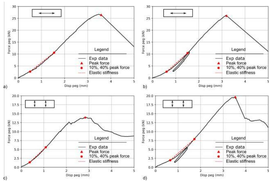
FIG. 14: Force-displacement experimental results of the column to beam connection via pegs.
