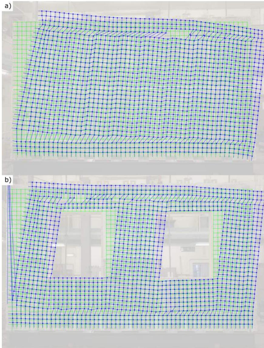
FIG. 6: Deformed shape at failure obtained by Digital Image Correlation for the a) SW\_noLoad specimen and b) WW\_noLoad specimen.
