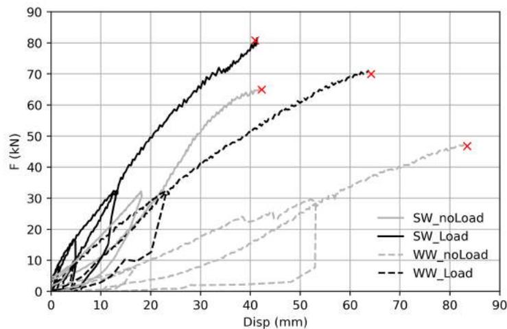
FIG. 4: Force-displacement response of the specimens.
