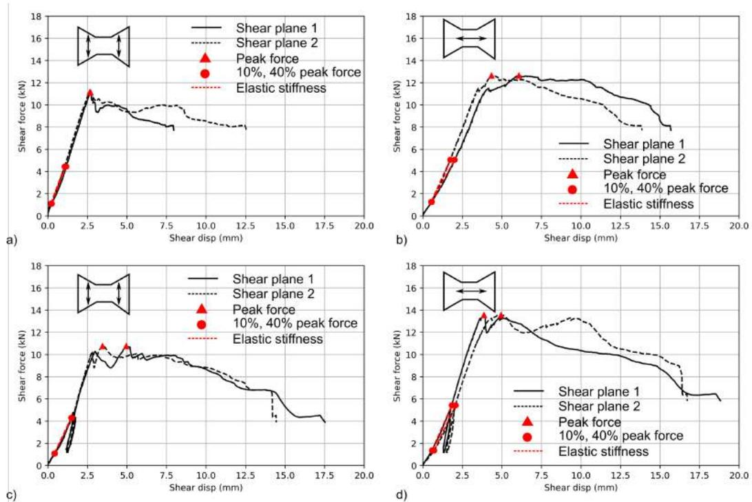
FIG. 9: Force-displacement experimental results obtained for each shear plane: a), c) monotonic and cyclic test on plywood specimens with 4 lamellae which grain is parallel to the shear plane; b), d) monotonic and cyclic test on plywood specimens with 2 lamellae in which the grain is parallel to the shear plane.
