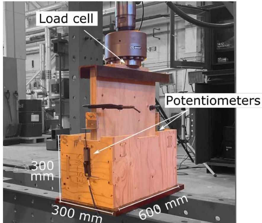
FIG. 12: Experimental setup to test the shear panel to column load path capacity (via pegs).
