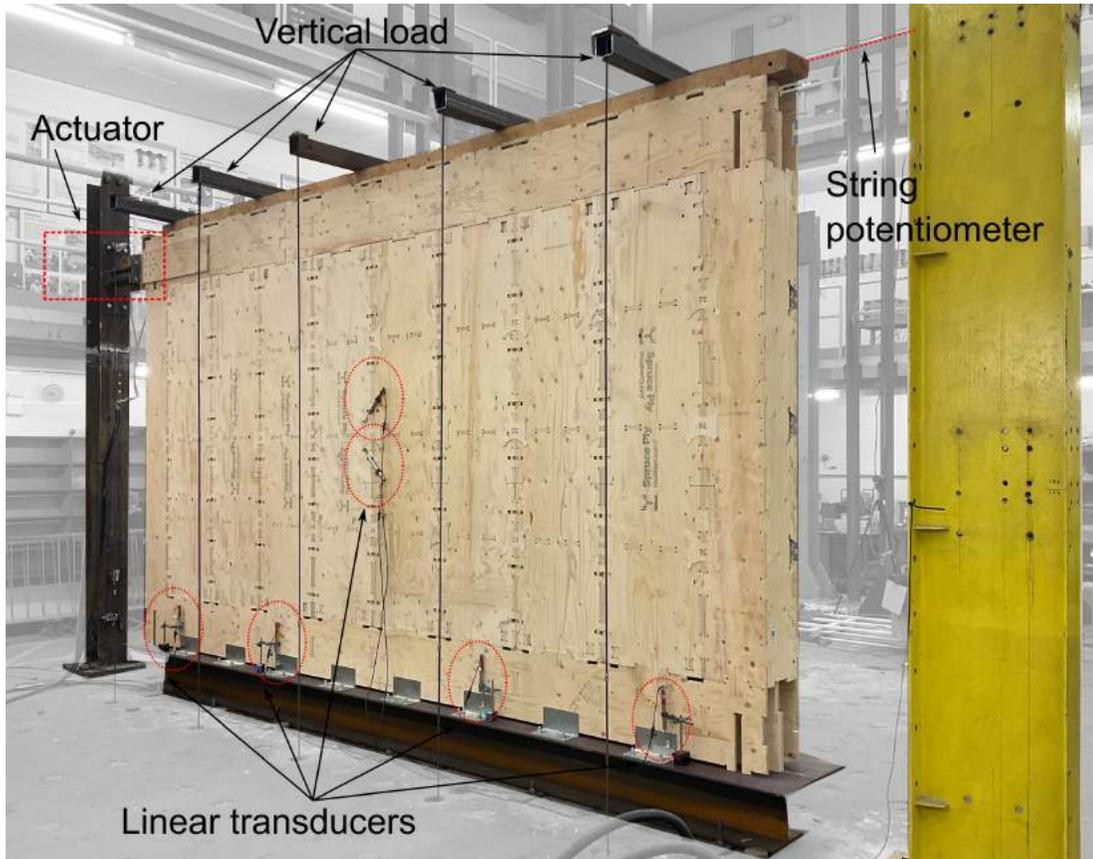
FIG. 3: Experimental setup for testing the walls.
