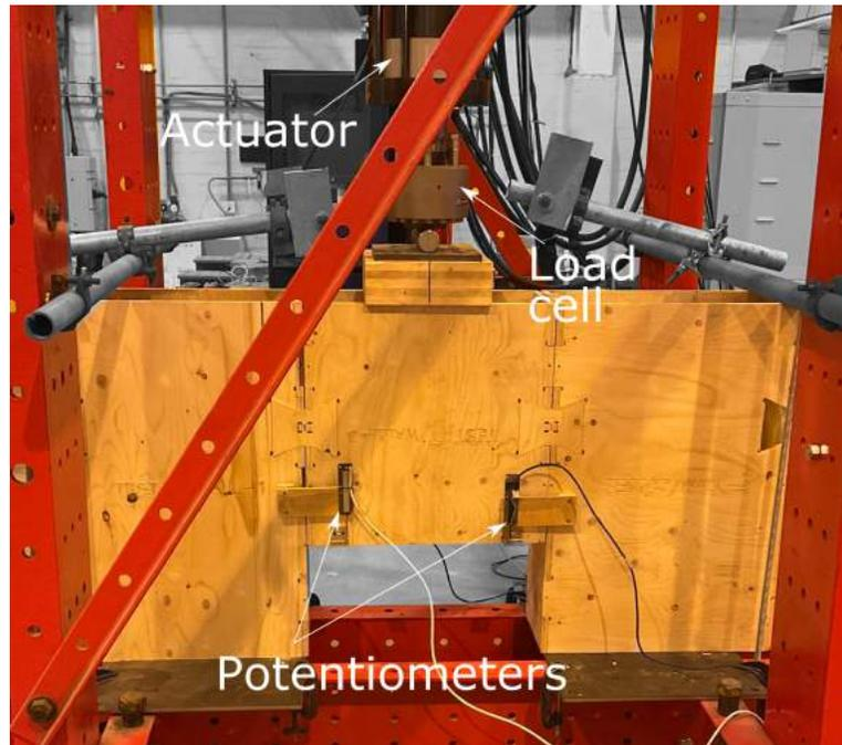
FIG. 7: Experimental setup to test the shear connectors.
