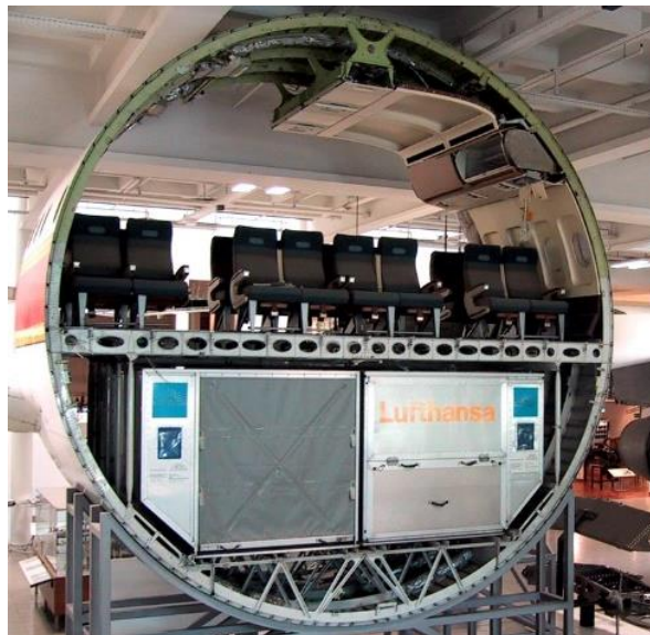
Fig. 1. LD3 containers loaded into an Airbus A300 (Wikipedia, NA).
