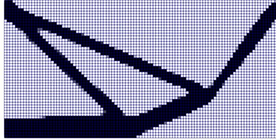
Figure 5: Topology optimization result for force inverter mechanism.
