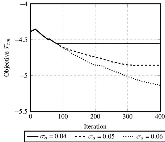
Figure 8: Evolution of compliant mechanism objective of force inverter when subjected to local stress constraint. The three lines correspond to different values of prescribed allowable stresses.
