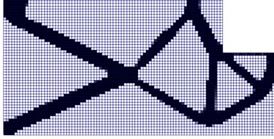
Figure 16: Topology optimization result for gripper mechanism.
