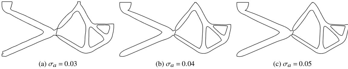
Figure 21: Optimized shape of gripper with global stress constraints in the domain
