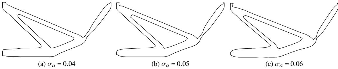
Figure 7: Optimized shape of force inverter with local stress constraints on the boundary. (a) Optimized for an allowable stress of 0.04 (b) Optimized for an allowable stress of 0.05 (c) Optimized for an allowable stress of 0.06.
