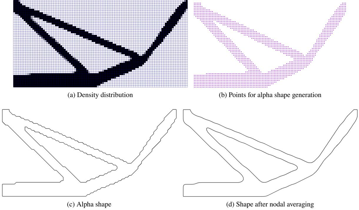
Figure 2: Steps involved in shape generation: (a) Density distribution after topology optimization (b) Centers of solid cells for alpha shape generation (c) Alpha shape enclosing the given points (d) Alpha shape after smoothing by nodal averaging.
