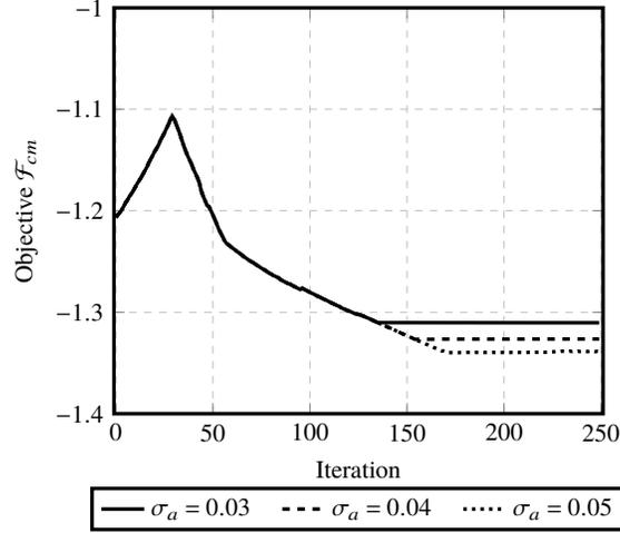
Figure 19: Evolution of compliant mechanism objective of gripper when subjected to local stress constraint
