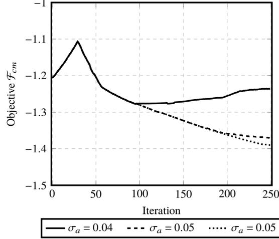
Figure 22: Evolution of compliant mechanism objective of gripper when subjected to global stress constraint
