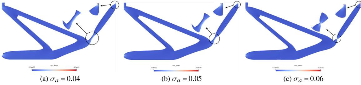
Figure 14: Stress distribution in force inverter subjected to global stress constraint.
