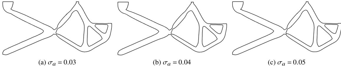
Figure 18: Optimized shape of gripper with local stress constraints on the boundary
