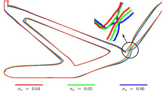
Figure 13: Comparison of design evolved for different allowable stress values with global stress constraint.
