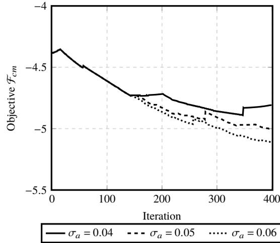
Figure 12: Evolution of compliant mechanism objective of force inverter when subjected to global stress constraint
