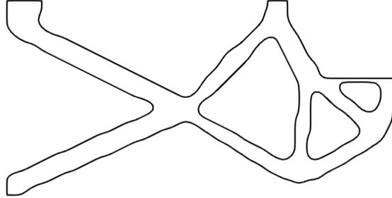
Figure 17: Shape generation of gripper mechanism from the result of topology optimization in Fig. 16.
