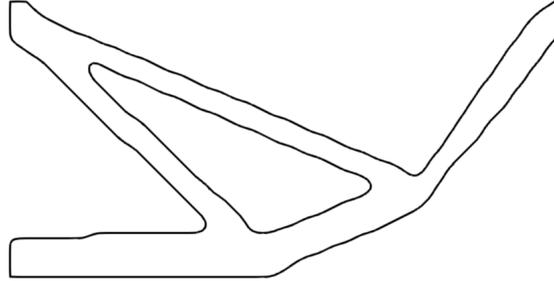
Figure 6: Shape generation of force inverter from the result of topology optimization in Fig. 5.
