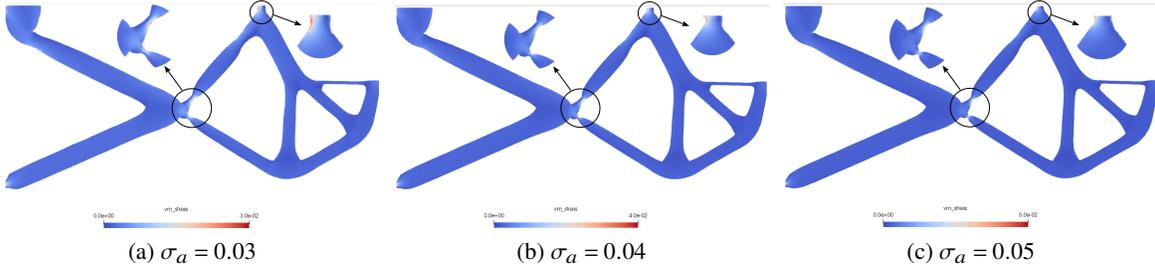
Figure 20: Stress distribution in gripper optimized subjected to local stress constraint
