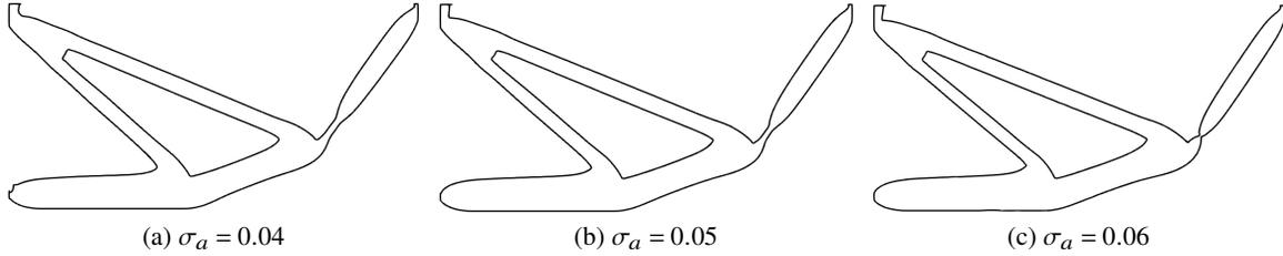
Figure 11: Optimized shape of force inverter with global stress constraints in the domain
