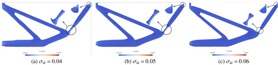
Figure 10: Stress distribution in force inverter subjected to local stress constraint
