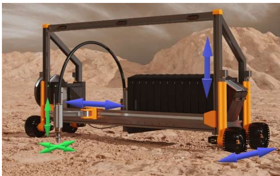
Figure 3 – Coarse positioning (Blue) and Fine positioning (Green) work together to allow precision printing over workspaces spanning 10's or even 100's of meters
