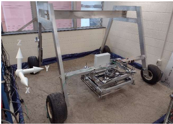
Figure 6 – Mud Dauber is a first generation prototype of the mobile gantry architecture.
