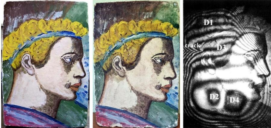
**Fig. 3.** The fresco model in 2000 (left), in 2022 (center) and inspected by holographic interferometry with defects position shown.
