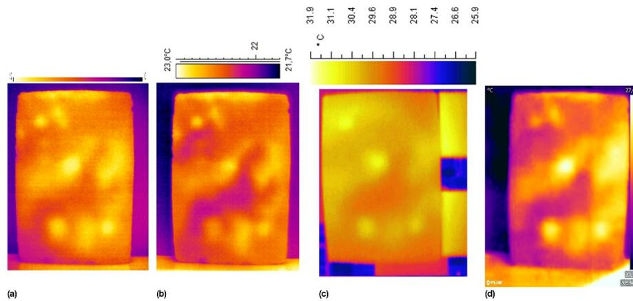
**Fig. 6.** Experimental results on the fresco model, obtained by the different thermal cameras, are presented. (a) FLIR T1020; (b) FLIR S65 HS; (c) AVIO TVS-2000MkII; (d) FLIR One.
