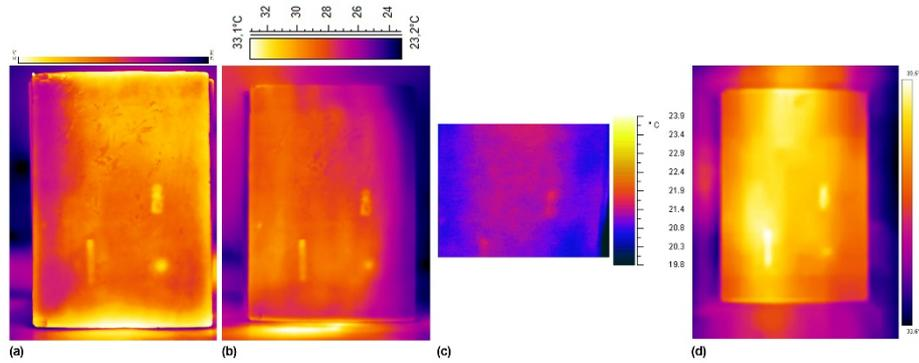
**Fig. 5.** Experimental results on the wooden painting, obtained by the different thermal cameras, are presented. (a) FLIR T1020; (b) FLIR S65 HS; (c) AVIO TVS-2000MkII; (d) FLIR One.
