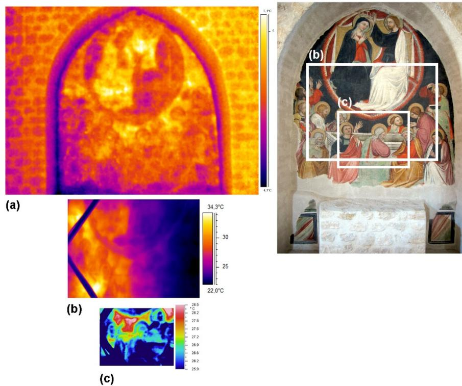
**Fig. 7.** Experimental results on a real case, obtained by the different thermal cameras, are presented. (a) FLIR T1020; (b) FLIR S65 HS; (c) AVIO TVS-2000MkII.
