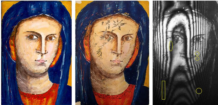
**Fig. 2.** The wooden painting model in 2000 (left), in 2022 (center) and inspected by holographic interferometry with defects position shown.
