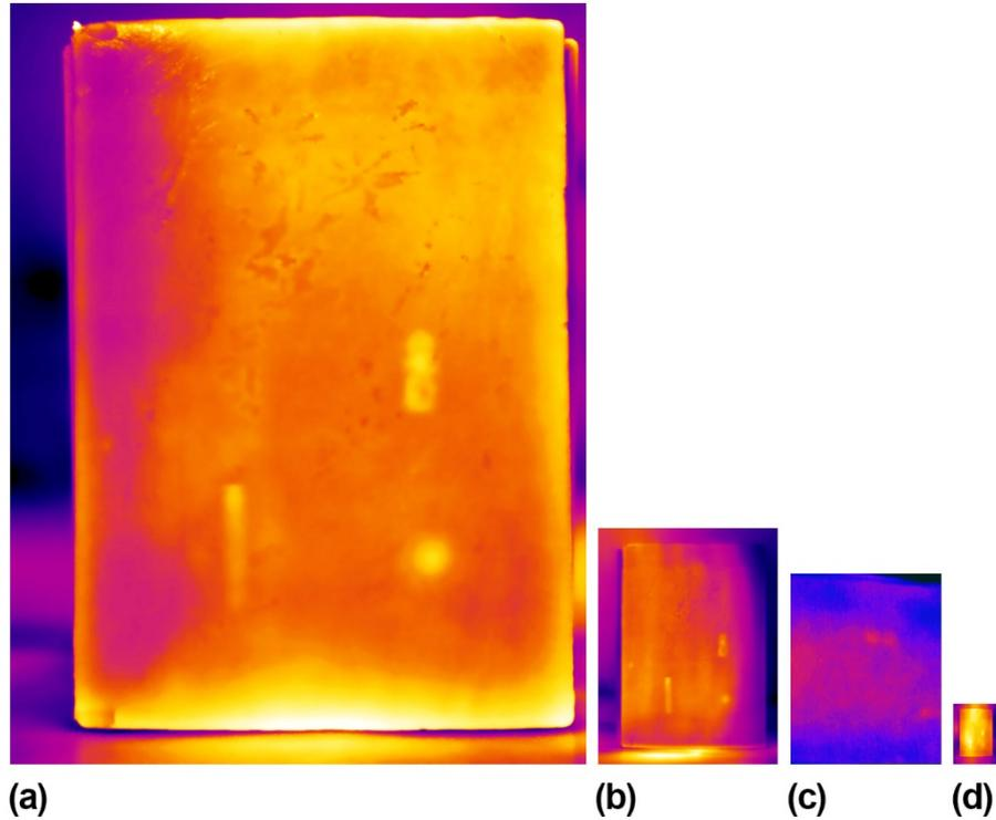
**Fig. 4.** Experimental results on the wooden painting, obtained by the different thermal cameras, are presented. Images dimensions are proportional to the resolution of the devices. (a) FLIR T1020; (b) FLIR S65 HS; (c) AVIO TVS-2000MkII; (d) FLIR One. For ease of comparison, (c) is rotated of  $90^\circ$  counterclockwise.
