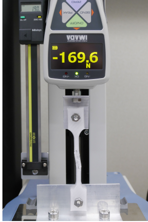
Figure 2: Tensile test of 3D-printed Okkake Daisen Tsugi (4.8 mm width)
