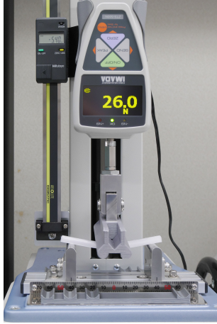
Figure 5: Bend test of 3D-printed Okkake Daisen Tsugi (4.8 mm width)
