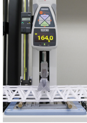
Figure 12: Bend test of a 3D-printed space frame ( 50/\sqrt{2} mm)
