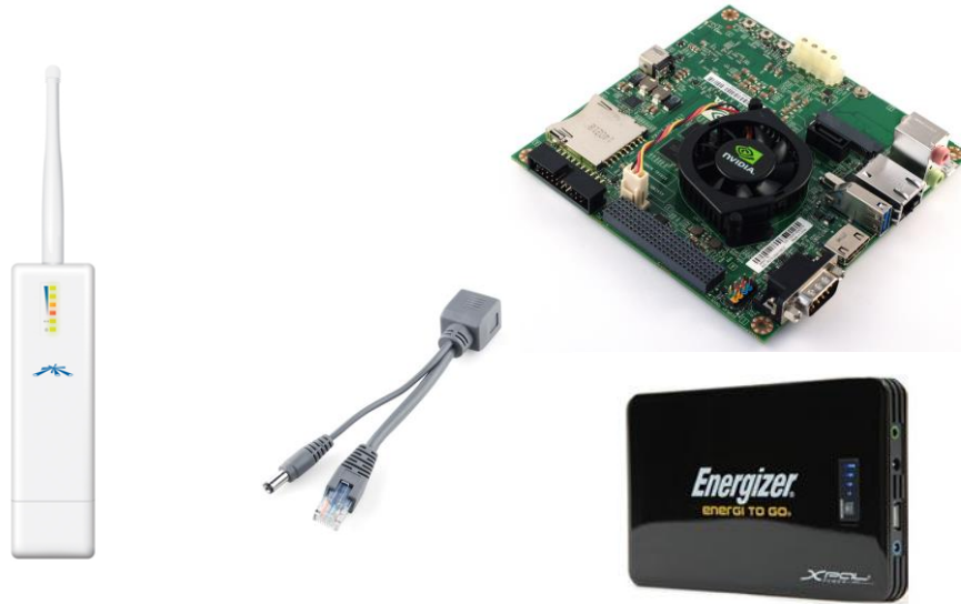
Fig: The wifi router was connected to the TK1 and Energizer via a power-over-Ethernet cable
