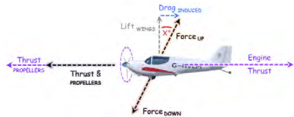
Fig. 5a-ii. Key forces acting on an airplane.
