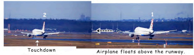
Fig. 10i-i. Ground effect observed on landing.
