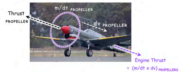
Fig. 5b-iii. Thrust generation by a propeller. [19]
