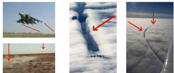
Fig. 4b-iii. Downwash evident behind airplanes.
