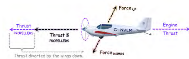
Fig. 5a-i. Key forces acting on an airplane in level flight.
