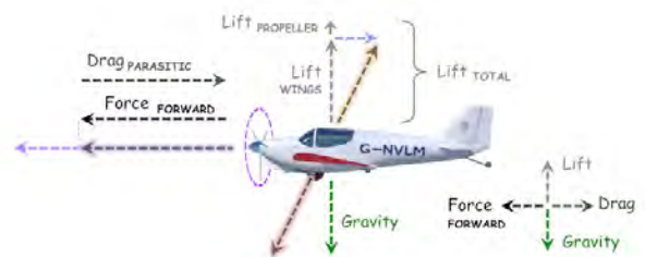
Fig. 5a-iii. Forces acting on an airplane defined by the two axis.
