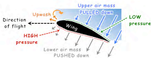
Fig. 6a-ii. 2D diagram of actual wing airflows. (Absolute airflow analysis.)
