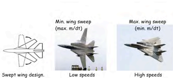
Fig. 10f-i. Variable wing-sweep wing design.
