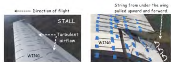
Fig. 7a-ii. Actual wing airflows in a stall.
