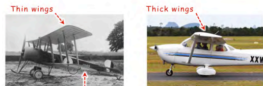
Fig. 10d-i. Old and modern airfoils compared. [19]
