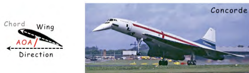
Fig. 10h-i. Delta-wing aircraft landing at high AOA. [19]
