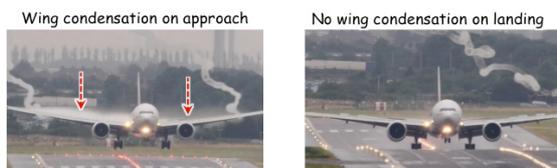
Fig. 4f-iii. Wing condensation on approach. [20]
