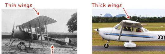
Fig. 4n-ii. Airfoils of old and modern wings compared.
