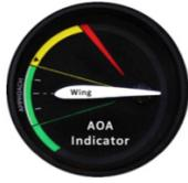
Fig. 10c. Example of an AOA indicator.
