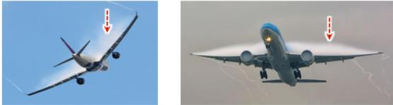
Fig. 4f-i. Wing condensation on airliners. [17][18]
