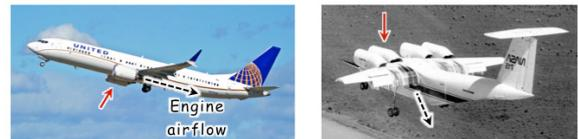
Fig. 4d-ii. Engines boost lift.
