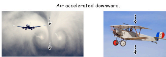
Fig. 10g-i. Wings accelerate air downwards. [14]
