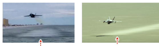
Fig. 4b-v. Pressure impulse below jets. [23]
