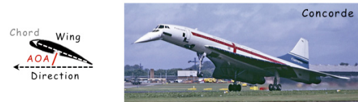
Fig. 10h-i. Delta wing aircraft landing at high AOA. [14]
