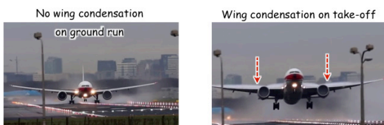
Fig. 10k-ii. Wing condensation on take-off. [20]
