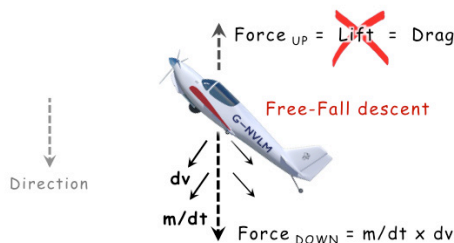
Fig. 7a-vi. Drag on an airplane in a free-fall descent.
