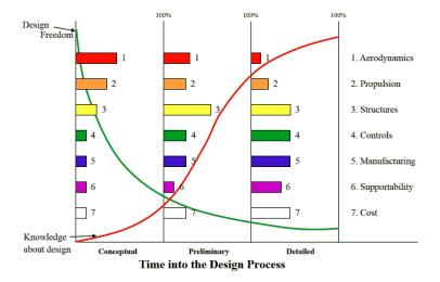
Figure 1: Uneven distribution of knowledge in the aircraft design process [24]
