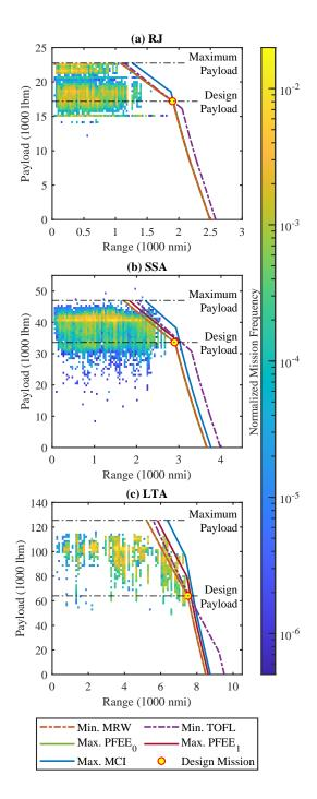
Figure 8: Payload-range envelopes of the single-objective optima
