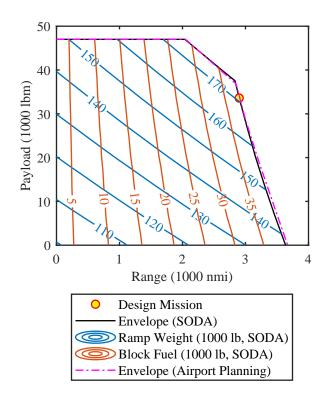
Figure 5: Comparison of payload-range characteristics between SODA outputs and Airport Planning data for a notional SSA resembling the Boeing 737-800
