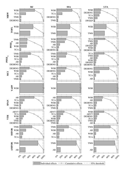
Figure 6: Normalized individual and cumulative effects of filtered effective design variables for individual responses
