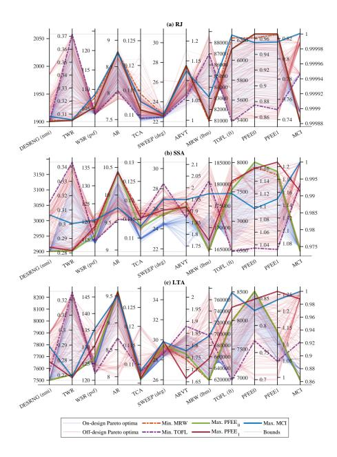
Figure 7: Design variables and objectives for Pareto optimal designs
