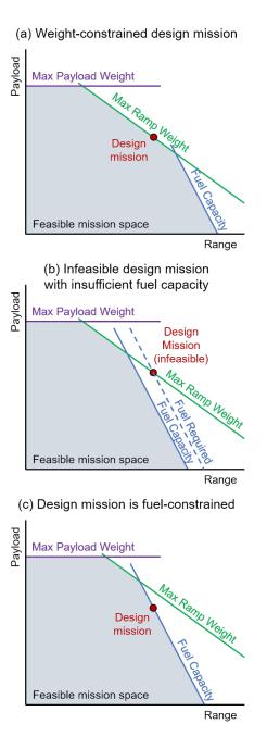
Figure 3: Notional payload-range diagrams for weight-constrained and fuel-constrained sizing
