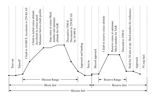
Figure 2: Generic mission profile for commercial aircraft
