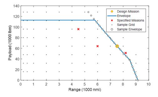
Figure 4: Notional payload-range diagram showing all mission types evaluated
