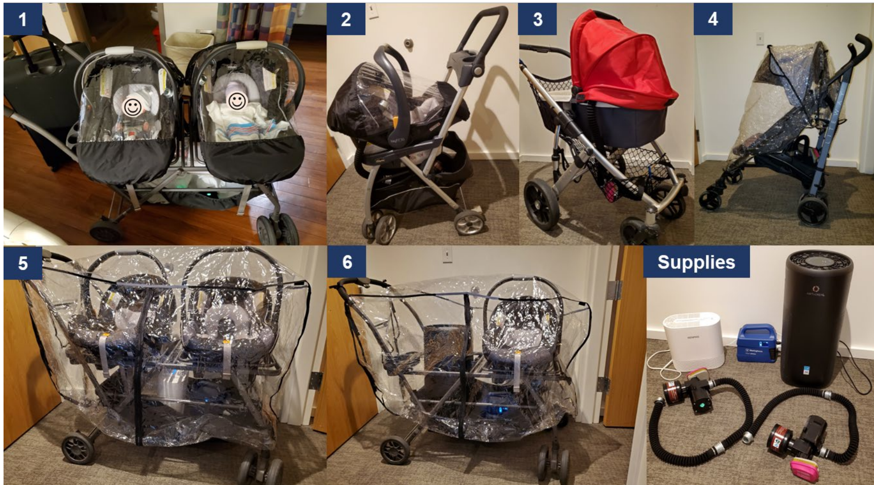
Figure A1. Case Prototypes of PAPR Buggies (Top Row) and HEPA Buggies (Bottom). Model 1: Twin children in individual covered car seats, each with separate PAPR devices. Model 2: Single child version for a covered car seat with PAPR device. Model 3: Bassinet stroller with PAPR device, requires cover, not shown. Model 4: Single seated stroller, covered, with PAPR device. Model 5: Two car seats with large cover, using a small HEPA attached to a portable power station. Model 6: Single car seat attached to a twin stroller frame with large cover, using a large HEPA and power station. Supplies shown include small and large HEPA filters, the portable power source, and two PAPR devices, each shown with a manufacturer’s P100 filter (brown) and 3M version (pink).
