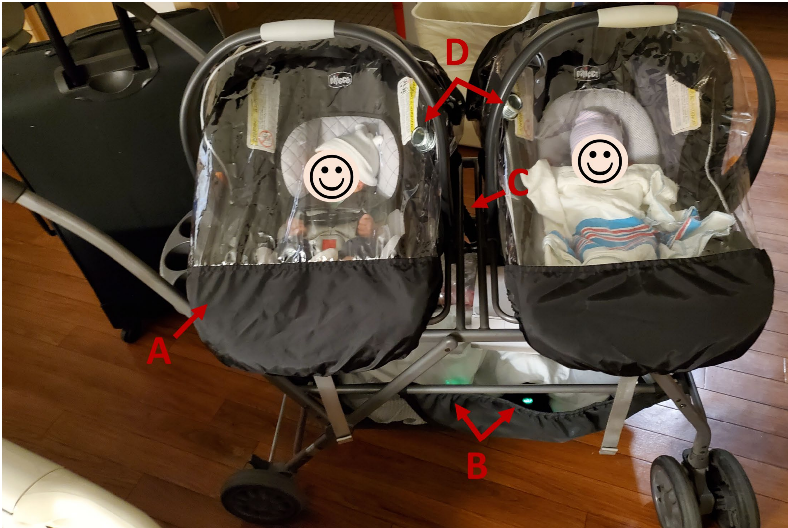
Fig 1. First Test-Run of a PAPR-Buggy to Improve COVID-19 Safety (Model 1 of 6 Tested). In this model, two car seats are covered individually with safe commercially-sold rain covers (A). A PAPR air-cleaning device for each child sits in the stroller's undercarriage (B), with the non-filter portions hidden by a muslin blanket. The black PAPR tubes discretely ascend the stroller frame (C) and tuck into the rain covers (D) to release fresh air. Six models were tested for 1-2 children using various strollers, rain covers, and PAPR/HEPA filters. The investigator's twins tested the models, starting with their first trip home from the hospital, pictured.
