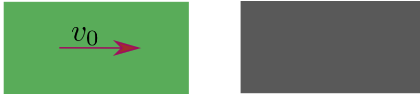
Figure 7: Collision between two rectangular elastic solids, where, the left solid is allowed to move towards the right solid with a constant velocity v_0 , while the right solid is at rest.
