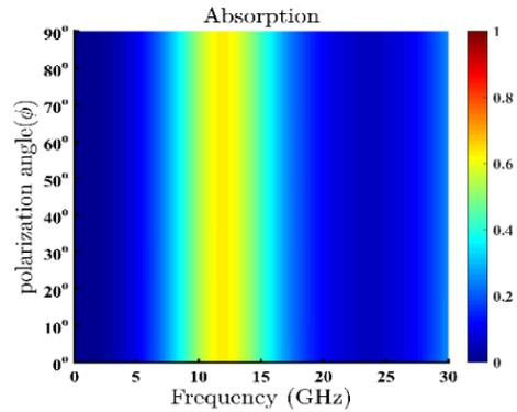
Figure 3. Polarization insensitivity analysis for the designed absorber
