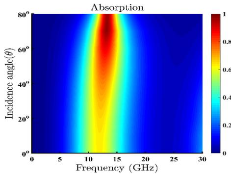
Figure 4. TE wave incidence angle analysis for the designed absorber
