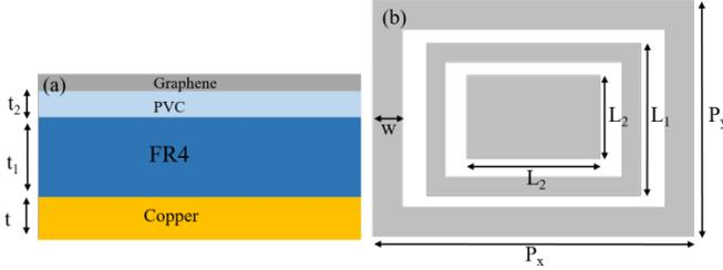
Figure 1. Unit cell of the absorber (a) Layered view, (b) Top view
