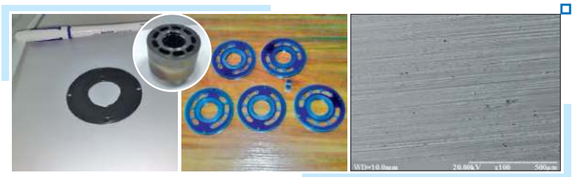
Fig. 3.57 Parts of aircraft units coated with molybdenum disulfide
