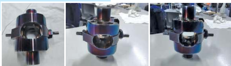
Fig. 4.3 Hydraulic units cradles with Avinit C310 nanocoating
