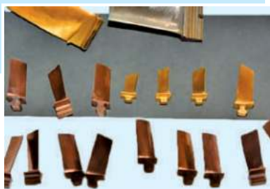
□ Fig. 3.29 Avinit C350 coating based on (Ti-Al-N)
