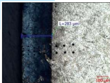
Fig. 3.39 Imprints of microhardness measurements (etched polished)
