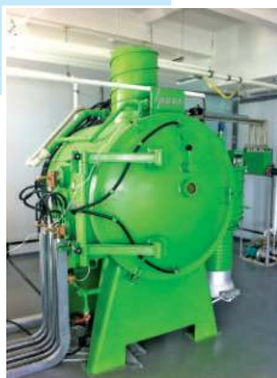
□ Fig. 4.9 One-chamber vacuum automated installation of diffusion welding and heat treatment of parts
