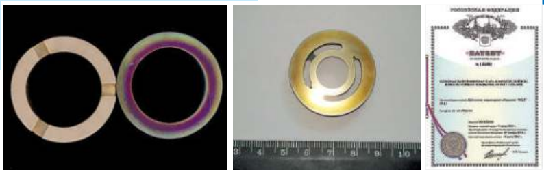
Fig. 4.4 Slide valves of hydraulic units coated with Avinit C320 [21–24]
