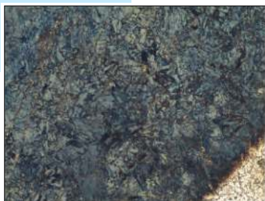
■ Fig. 3.36 The microstructure of the nitrided layer on 34NiCrMoV14-5 steel ( \times 500 )
