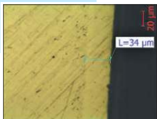
Fig. 3.12 Microstructure of Mo coatings
