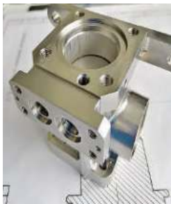
Fig. 3.53 Housing from DIN 3.7165 titanium alloy. The structure of the nitrided layer on the inner cylindrical part of the housing surface
