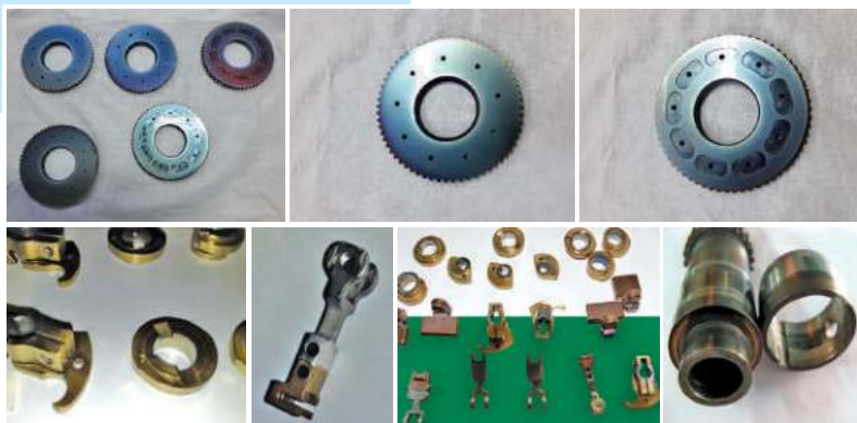
Fig. 4.2 Parts of Avinit C310 serial aviation hydraulic units with nanocoating
