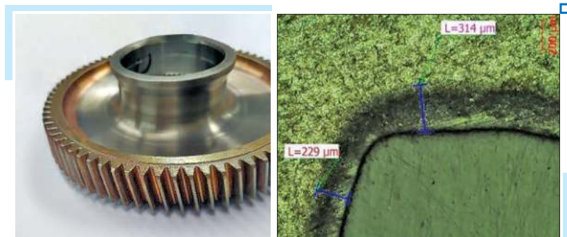
Fig. 3.49 Plasma nitriding of Avinit N steels 34NiCrMoV14-5. Depth of the nitrided layer 0.3 mm. Microhardness H_{\mu}=730\text{--}930
