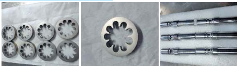
Fig. 4.6 Serial parts of aviation hydraulic units, nitrided by plasma precision nitriding
