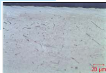
Fig. 3.46 Nitrided layer from side No. 2, \times 500
