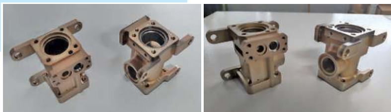
■ Fig. 4.8 Serial nitriding of titanium DIN 3.7165 housings
