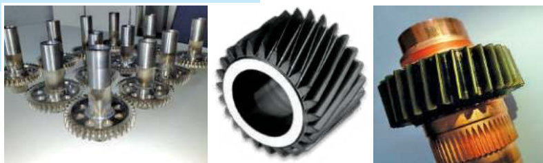
■ Fig. 4.7 Serial nitriding of gear wheels (34NiCrMoV14-5)
