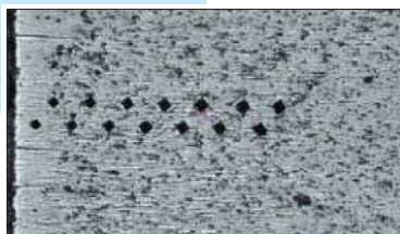
Fig. 3.47 The microhardness measurements imprints. Side No. 1
