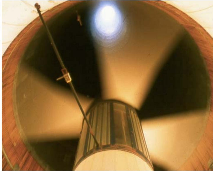
FIGURE 1.2: Manzanares prototype turbine [4].
