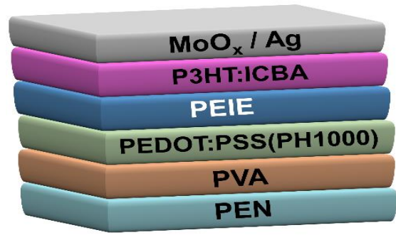
Fig. 1. Schematic of various participating layers of organic photovoltaic (OPV) device.
