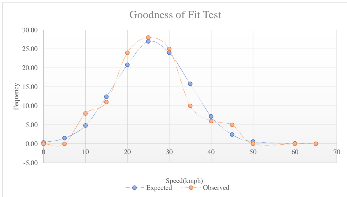
Figure 14: Goodness of the Fit Comparison with theoretical and corrected observed value
