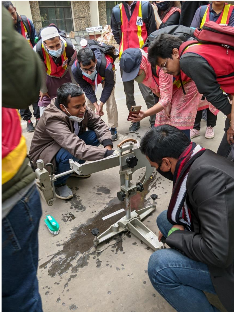
Figure 9: Skid Resistance being Tested
