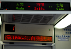
Onboard information system (top) from a newer EMU700 identifies prior stop (Wudu), next stop (Baifu), and following stop (Qidu); flexible scrolling display from older push-pull sets are similar to platform displays (bottom).
