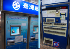
Advance-purchase ticket machines have touch screens, reservations, and credit card capabilities (left); commuter ticket machines are simple and robust prepaid-card and cash-only receipt printers (right).
