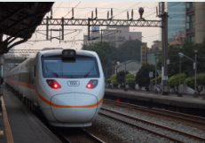
TRA purchased six sets of Hitachi 8-car 130 km/h tilting trains, based on JR Kyushu's 885-series design, for US$85 million, to provide accelerated East Coast services. Locally called "Taroko trains" after the mountain gorge.
