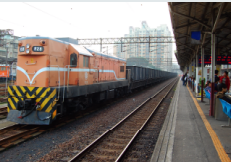
An empty coal train with an American Electro-Motive Division (EMD) G12 (TRA R20-class) locomotive is stored on Taoyuan's bypass track, likely recently returned from the Linkou coal-fired power plant.
