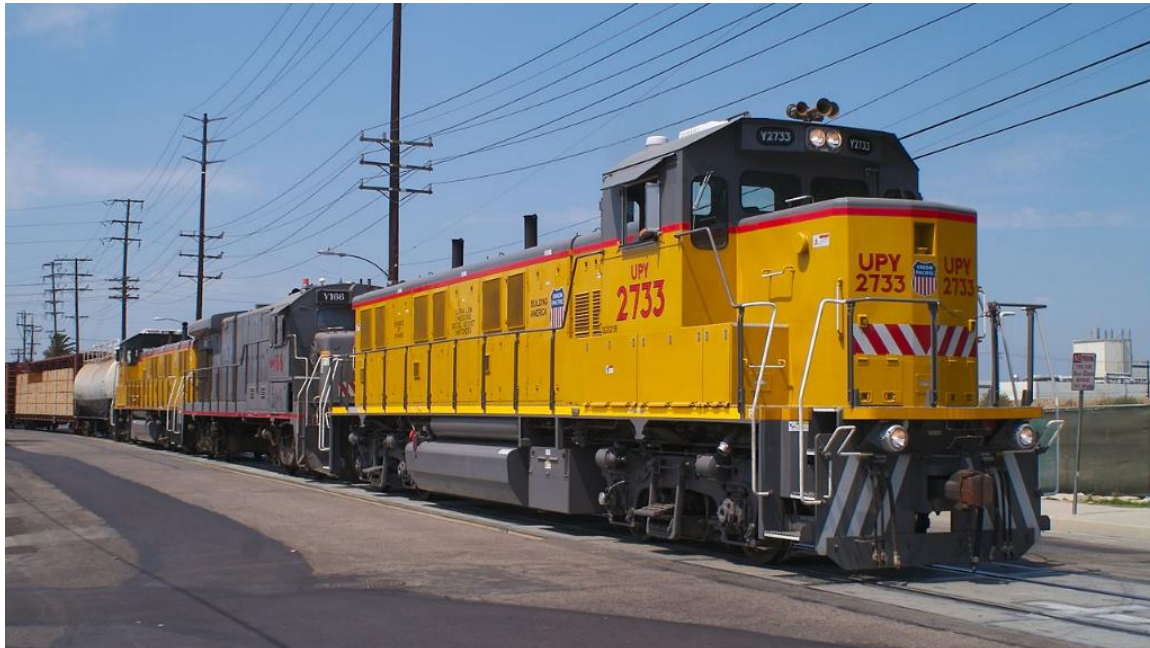
Figure 4. NRE 3GS21B, a popular “genset” locomotive, on Olive St., Anaheim, California, 2007; Matthew “Morven” Brown photo (CC BY-SA 3.0). ( https://commons.wikimedia.org/wiki/File:NRE_3GS21B_UPY_2733.jpg )
