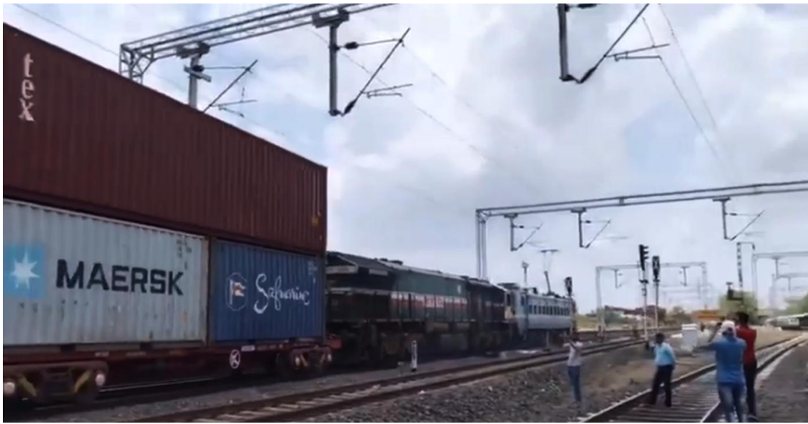
Figure 14. On Indian Railways, the Western Railway operates this electrified double-stack container train from Palanpur to Botad in Gujarat, June 10, 2020; Piyush Goyal photo (Government of India Open Data License via http://indianrailways.gov.in/ ).
