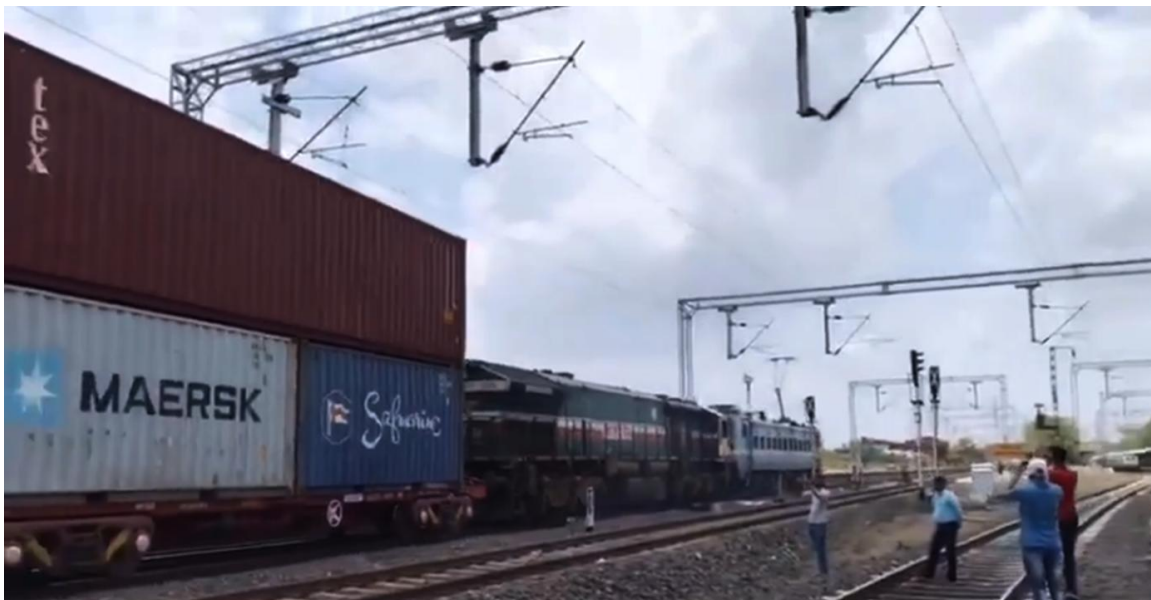
Figure 17. On Indian Railways, the Western Railway operates this electrified double-stack container train from Palanpur to Botad in Gujarat, June 10, 2020; Piyush Goyal photo (Government of India Open Data License via http://indianrailways.gov.in/ ).
