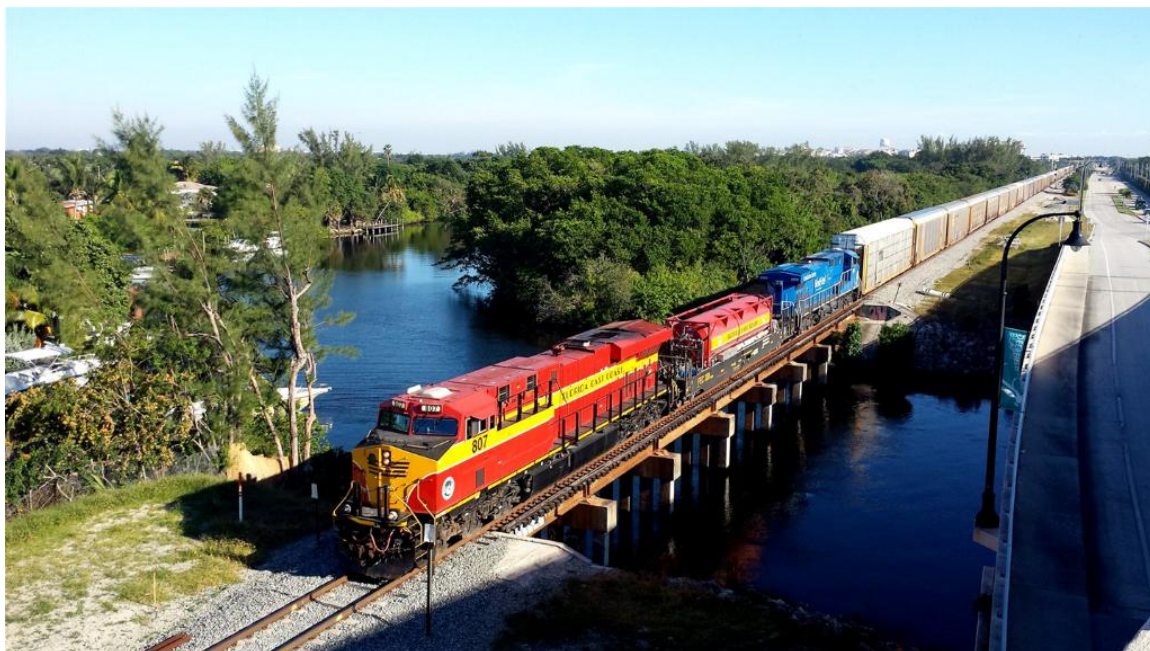
Figure 3. Florida East Coast Locomotive 807 and Liquefied Natural Gas (LNG) Fuel Tender 302 at the Dixie Overpass, Deerfield Beach, Florida. Flickr User BBT609 photo (CC BY 2.0). ( https://www.flickr.com/photos/bbt609/30873507632/ )
