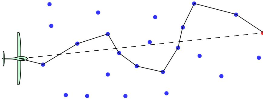
**Fig. 7** Path planning for a pilot in the risk minimization frame. The pilot will fly to the nearest thermal option (in blue) which brings the pilot nearer to the next turnpoint (red). The pilot will accept large deviations to minimize the distance which must be flown before encountering a potential thermal.
