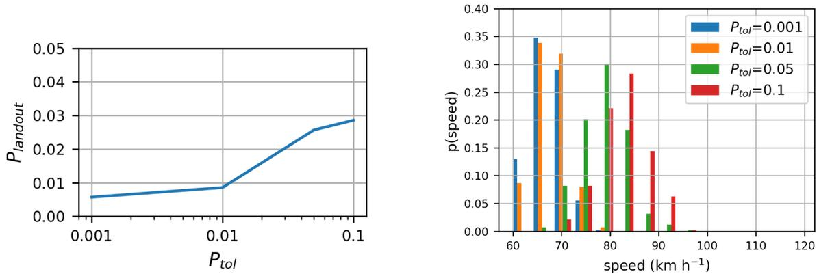
(a) Probability of failing to complete a task when the probability that a given thermal works is 0.4 and the pilot can shift gears. The horizontal axis is plotted on a log scale.
