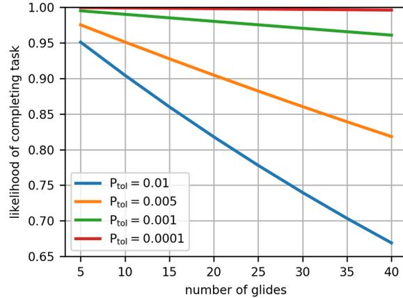
**Fig. 1** Probability of completing a task given the number of glides required. The completion probability is shown for several levels of risk tolerance on each glide. For long tasks, the probability of completion is very sensitive to the risk tolerance, and even seemingly low risk tolerances can result in a significant probability of landing out.
