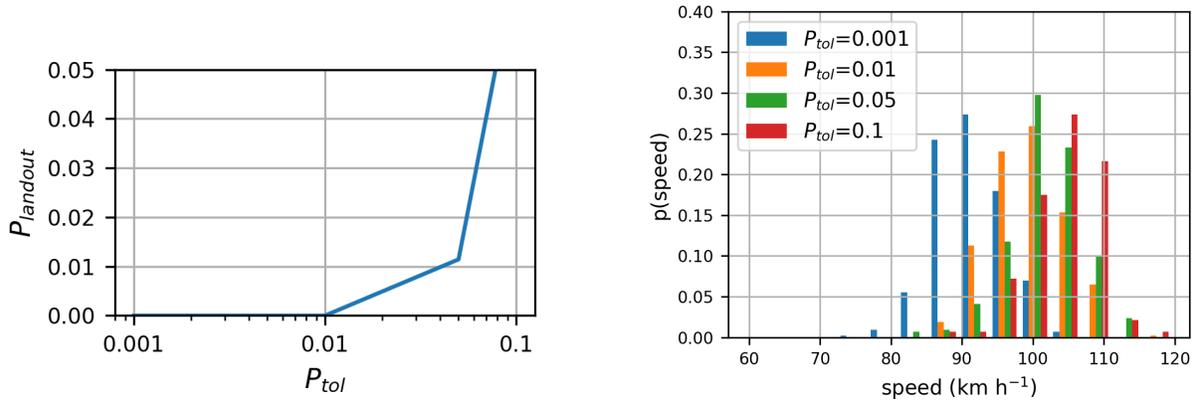
(a) Probability of failing to complete a task when the probability that a given thermal works is 0.7 and the pilot can shift gears. The horizontal axis is plotted on a log scale.
