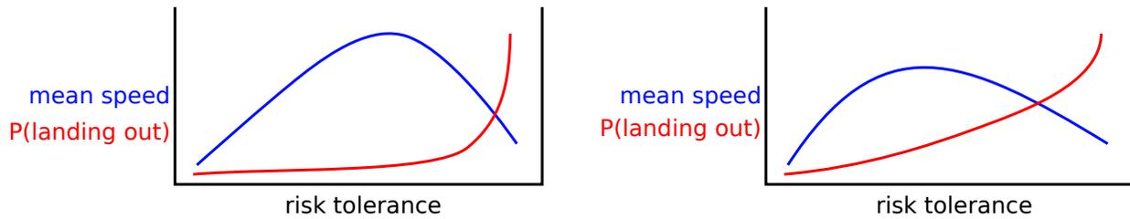
(a) In an environment which lightly penalizes risk, the pilot can initially be much more aggressive. We expect that this permits an initial behavior closer to the optimal speed while not exposing the pilot to too great a risk of landing out.
