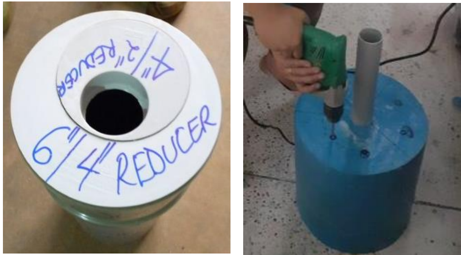
Figure 2: Using PVC diameter reducers in Uganda (left), drilling holes for tubing in Nepal (right).
