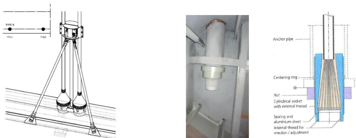
Figure 3 - Lower end of the hanger (left) and anchor pipe (right)
