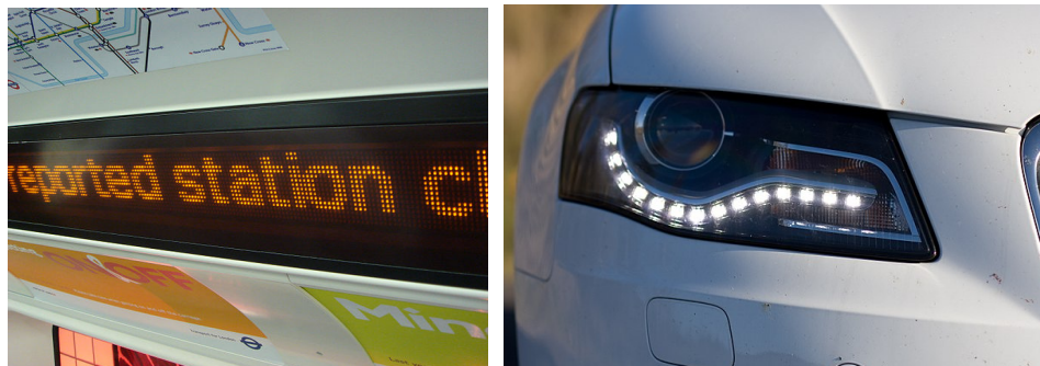
(a) LED display on London Underground. (b) Used as daytime running lights on vehicle.
