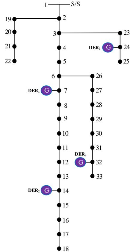
Fig. 4. The modified 33-node distribution system
